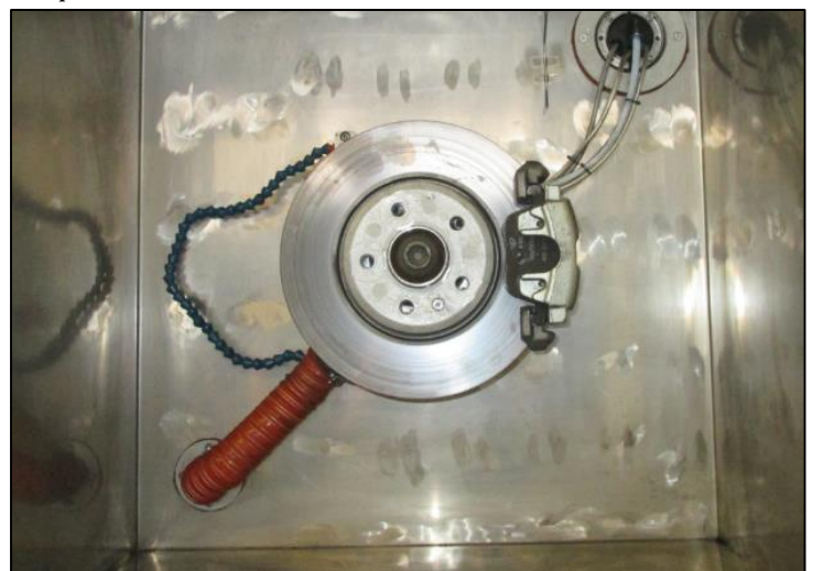
Drive axle inside the chamber (view on the break system)
