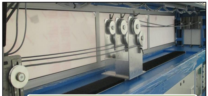
Installation of the Test specimens
