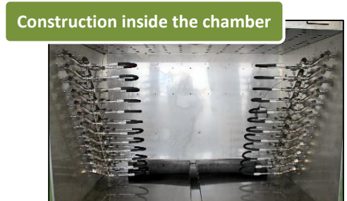
Adjustable distance from 150 mm to 450 mm
