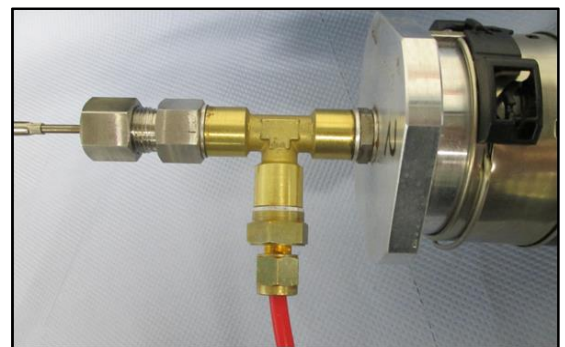
Test specimen connection (by means of copper capillary)
