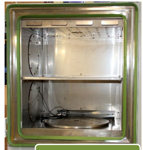
Test chamber inside
