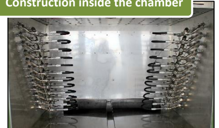
Adjustable distance from 150 mm to 450 mm
