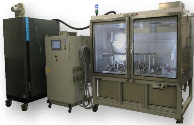
The test bench components (nitrogen generator / control unit / test cell)
