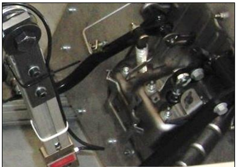
Mounting of the pedals in the test bench
