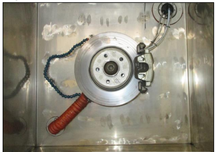
Drive axle inside the chamber (view on the brake system)
