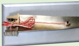
Strain gage application and measurements (application and calibration at various objects, e. g. circuit boards, turbine blades)
