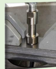
Special force transducer and calibration (Waterproof application with strain gage)
